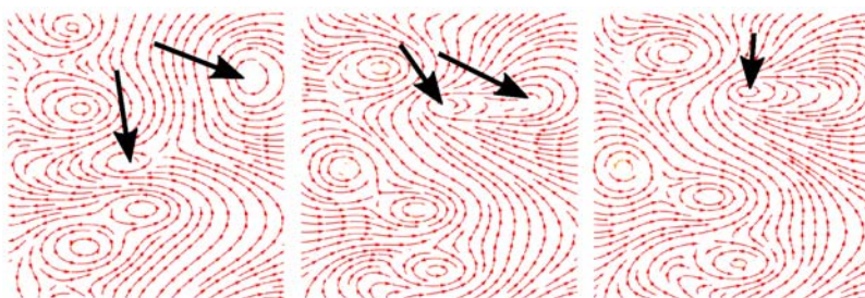
FIG. 12. Dynamical fusion with five rotors. Black arrows mark the two centers in the last frame combine into one. Flow fields are shown in (\theta, \phi) chart.
